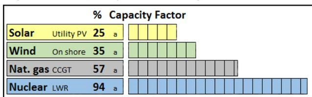
total cost per kWh. This graph depicts the average capacity factor for each source in the US in 2019. [a] The capacity factor of nuclear power plants was 3.8 times greater than solar, and 2.7 times greater than wind. This was primarily due to the intermittent nature of sunshine and wind.
